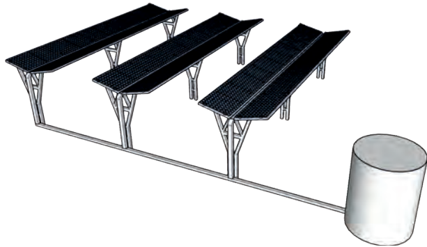
Fig. 55: Concept for a rain collection facility with storage tank © Fraunhofer ISE
